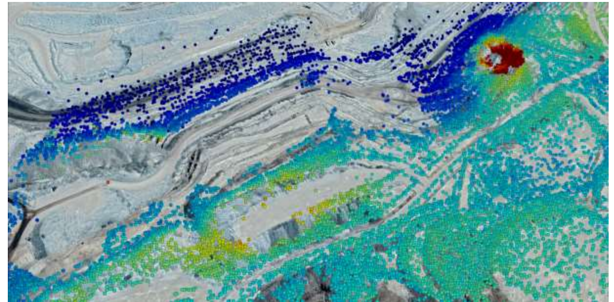
PSI deformation map showing points colorized by deformation rate at Rossing Uranium Mine in Namibia. One location (red) shows significant and continuous deformation on the steeply sloped edge of the mine.
